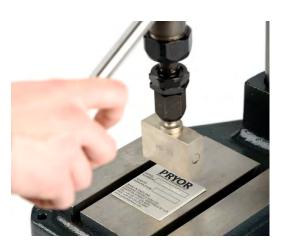
Press Holders and Shanks for use with Interchangeable Steel Type are available for Press marking to allow faster throughput.
